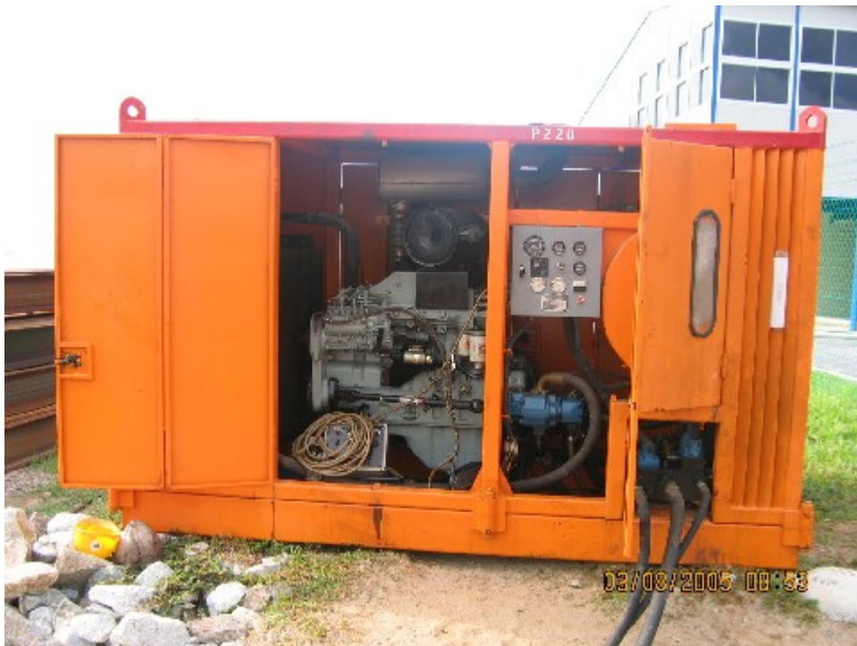
Vibro-driving: Power pack for vibro hammer
